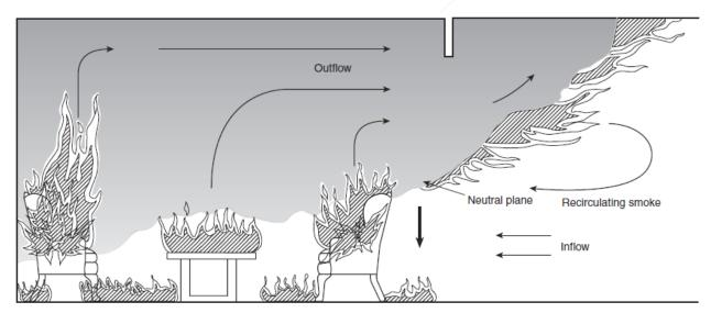
Figure 4. Flashover conditions in a compartment fire.
