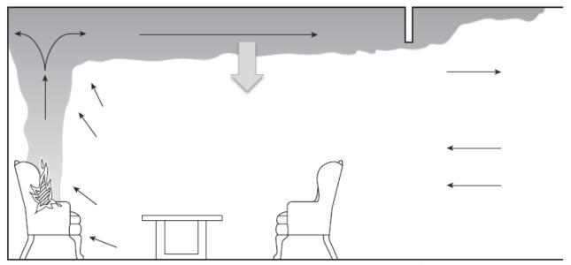
Figure 2. The enclosure smoke filling stage of an enclosure fire.
