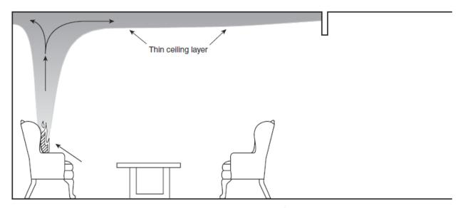
Figure 1. The fire plume/ceiling jet stage of an enclosure fire.
