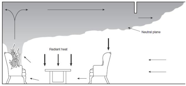
Figure 3. The pre-flashover vented stage of an enclosure fire.
